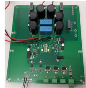
Developed board for packaged device dynamic characterization
